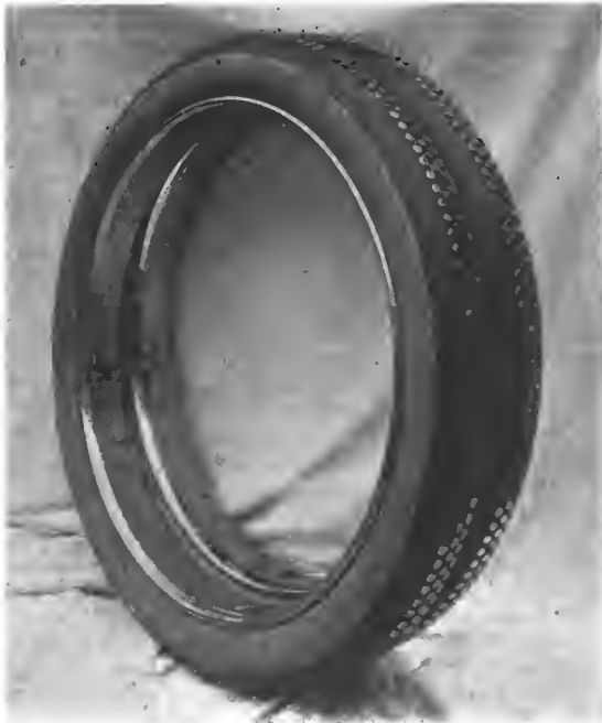
Showing the Michelin Twin Tires When Dismounted.
